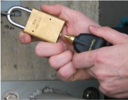
5. Use the CyberKey to contact each lock that requires updating. If access is not granted to the lock, the key will beep three times indicating a completed transaction.
